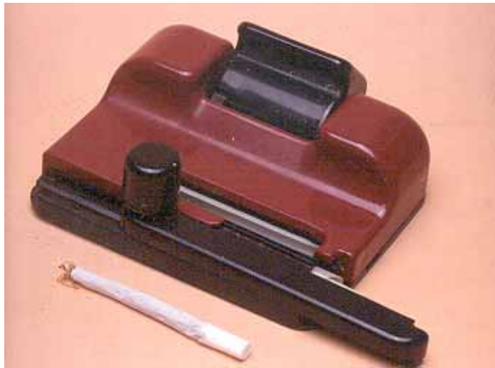
Figure 6. Rolling machine with stylus for inserting tobacco into empty tubes of cigarette paper.
